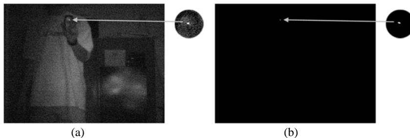
Figure 2. On the left, an unprocessed IR view captured by our camera detector with plenty of ambient light in the room. A person holds a camera phone pointed at a region in the environment we want to protect from capture. On the right is the processed view. The camera is detected by locating a bright white circular speckle.
