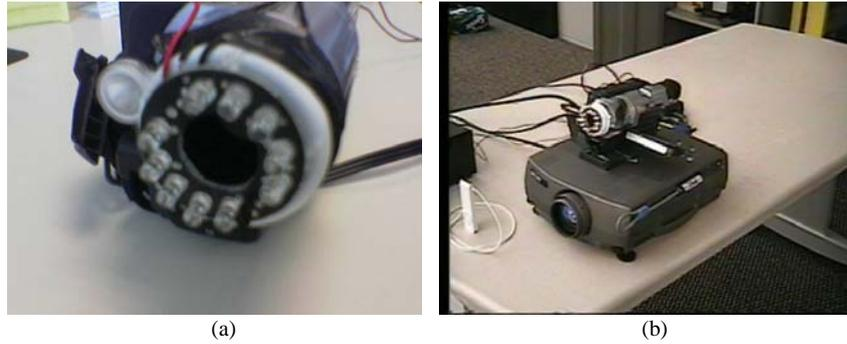
Figure 3. On the left shows our camera detector unit. We outfitted a Sony HandyCam, placed in *NightShot* mode, with a collection of IR transmitters and covered the lens with a narrow bandpass IR filter. On the right shows our camera detector coupled with a projector to neutralize cameras in the environment.
