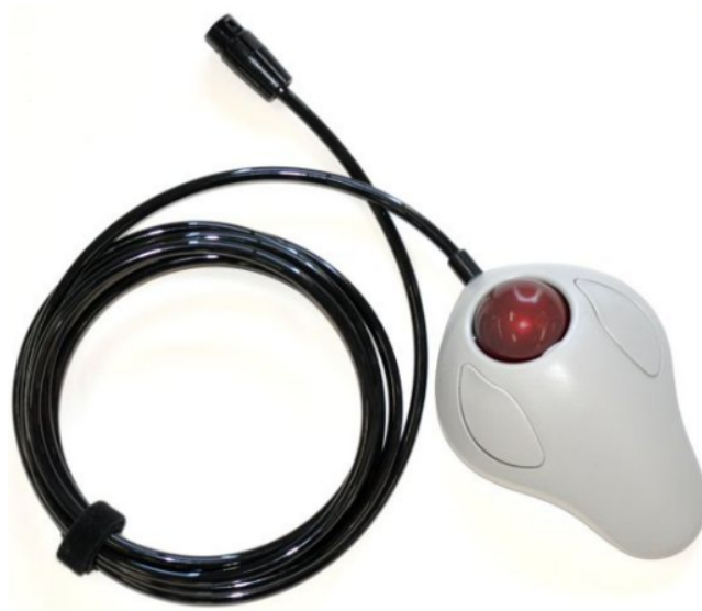
Figure 2: The Trackball 2 model from Current Designs is MRI safe, and constructed without metal. The connecting cable shown is a fiber-optic cable with 12 fibers. Not shown is a special interface that connects the fiber cable to a standard USB cable.
