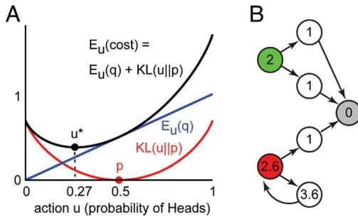
**Fig. 1.** New problem formulation. (A) A coin-toss example where the action corresponds to biasing the coin. The optimal bias is obtained by minimizing the sum (black) of the KL divergence cost (red) and the expected state cost (blue). Note that the tosses are independent and thus the temporal dynamics are irrelevant in this example. (B) A stochastic shortest-path problem illustrating how our framework can capture the benefits of error tolerance. See main text.
