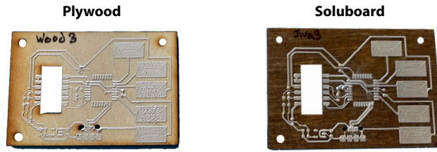
Figure 10: Material comparison. Circuit printed by the Voltera on plywood (left) and Soluboard (right).
