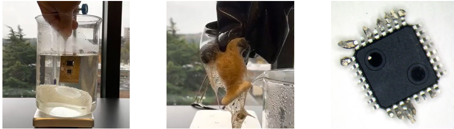
Figure 8: Component Reuse. Fully populated circuit and PVA mouse case being dissolved in hot water (left). The fibers and components can be recovered after dissolving (center). A recovered chip after baking in an oven to remove moisture is shown (right). This chip and a voltage regulator were successfully reused.
