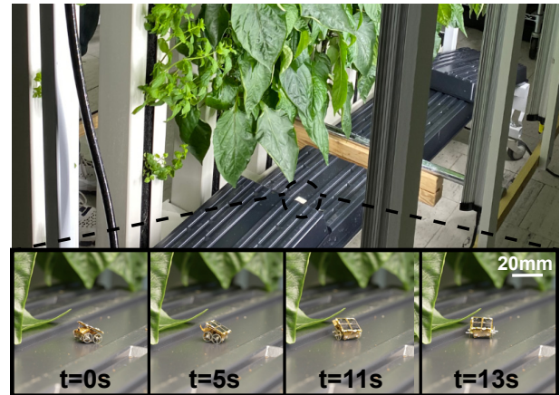
Figure 19: Battery-free and wireless MilliMobile operation at the bottom of a hydroponic farm. The solar cells onboard harvest power from nearby grow lights.
