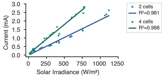
**Figure 13: Solar irradiance to current.** This plot shows current harvested from two and four solar cells at different light levels. We apply linear regression to obtain a mapping with  $R^2 > 0.98$  for both ( $N \geq 40$  measurements).
