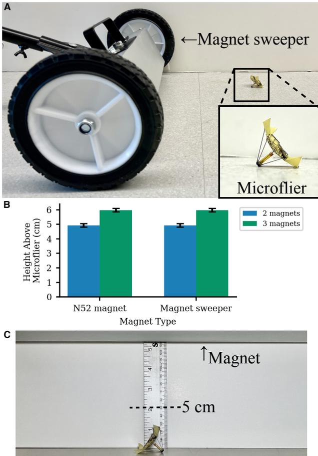
**Figure 16: Magnet pick up tests. A) Demonstration of automated microflieger pick up using a magnet sweeper. B) Average height that the microflieger is attracted to the pickup system using two different magnets ( $N = 10, \pm\sigma$ ). C) Test setup for data gathered in B).**
