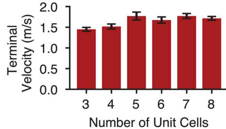
**Figure 17: Terminal velocity data. Average terminal velocity of the leaf-out design with three through eight unit cells when dropped in the tumbling state from a height of 2 m state ( $N \geq 10, \pm\sigma$ ).**
