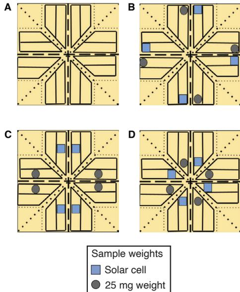
**Figure 10: Weight distribution tests.** We attach sample weights in different configurations to the origami structure simulating the mass of the solar cells and electronic components. We perform drop tests in each configuration to understand the effect of weight distribution on falling behavior.
