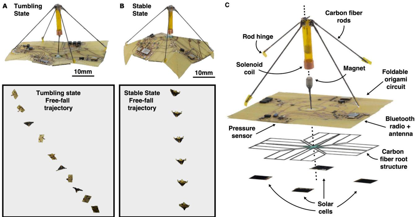
**Figure 2: Tumbling and stable states. A) Origami microflyer in its tumbling state. The free fall trajectory shows sampled video frames of the flipping and lateral motion. B) Origami microflyer in its stable descent state. The free fall trajectory shows stable descent and minimal lateral motion. C) Disassembled view of our origami microflyer showing the major components.**
