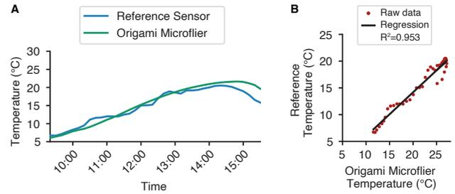
**Figure 15: Sensor evaluation.** A) Day long comparison of temperature sensor data from our deployed origami microflier and a reference sensor demonstrating a similar trend after a fixed offset subtraction to compensate for differences in placement and thermal mass of the reference sensor. B) Linear regression showing high correlation between the microflier sensor and the reference with  $R^2 > 0.95$  ( $N \geq 9000$  1 Hz measurements).
