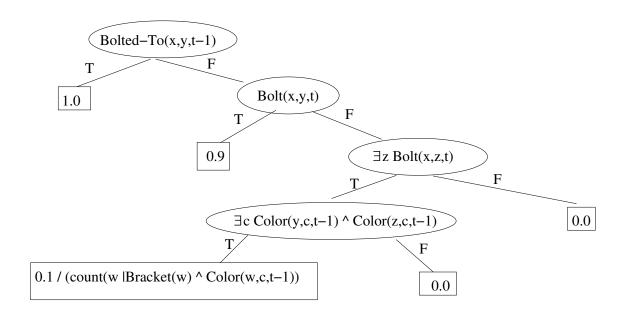
Figure 3: A first-order probability tree for the Bolted-To(x, y, t) predicate.
