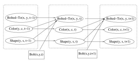
Figure 2: An RDBN representing the assembly domain.
