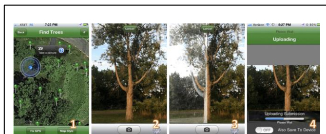
Figure 2: Workflow of the rePhoto app, (1) choosing, then (2) verifying the photograph subject, then (3) aligning the current camera view to match the previous picture, and (4) uploading the image.
