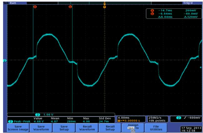
Figure 13: Plot of voltage across the terminals of the CFL with dimmer level set to 100.
