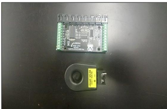
Figure 5: Phidgets Interface Kit and Current Detector.
