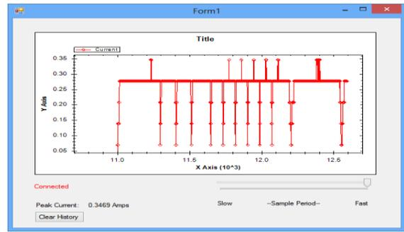
Figure 6: Real-time Plotting Utility Reporting Current Consumption.
