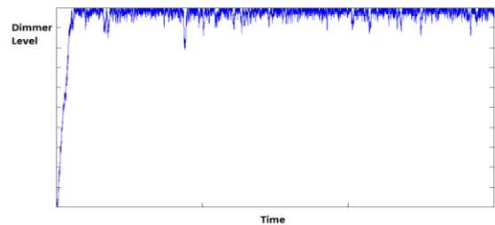
Figure 10: Random Gaussian distributed signal applied to CFL. Plot of Z-Wave dimmer level versus time.
