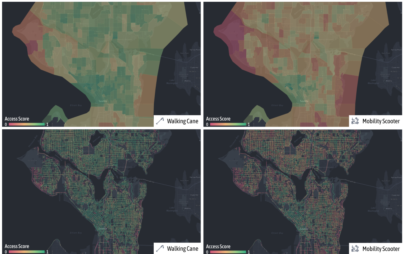
Figure 13: AccessScore maps visualizing sidewalk quality in Seattle for two groups: walking cane and mobility scooter (red is least accessible; green is most). Top two shows AccessScore by neighborhood; bottom two shows AccessScore by sidewalk segment. From the comparisons between walking cane users and mobility scooter users, we can see while downtown area may be equally accessible for both user groups, other areas are less accessible for mobility scooter users.
