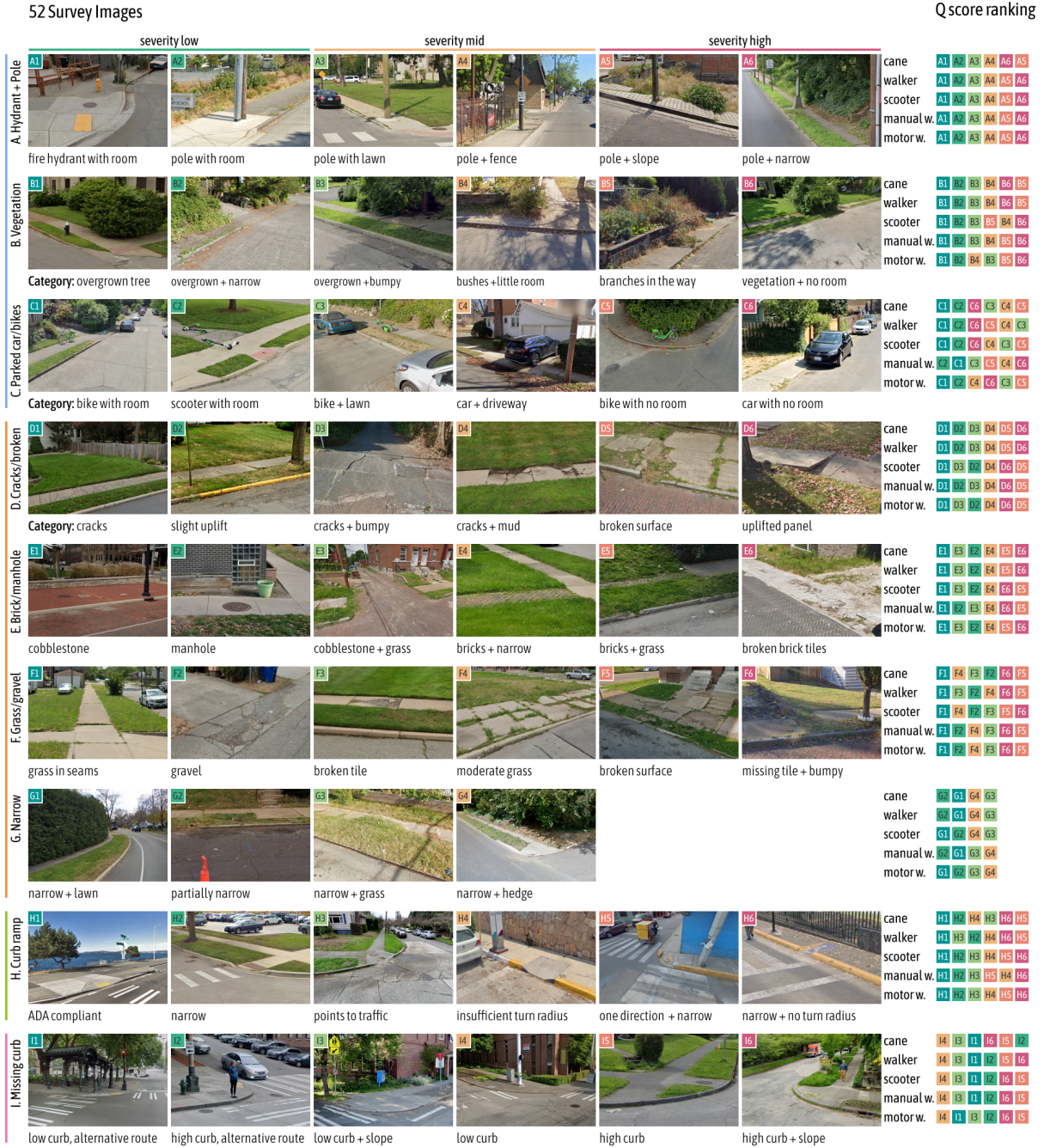
Figure 15: This figure presents 52 images used in the survey categorized into 9 sidewalk issue types (A-I). Each category contains 6 images, with 2 images per severity level (low, medium, high). The categories are further grouped into 4 Project Sidewalk label categories: Obstacles (A-C), Surface problems (D-G), Curb ramps (H), and Missing curb ramps (I). The matrix on the right displays the Q score ranking per user group for each category, arranged from the most passable (left) to the least passable (right).
