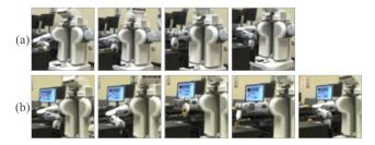
Fig. 6: Two programs that re-use abstracted procedures (opening the drawer and closing the drawer) (a) putting an object into the drawer, and (b) taking an object out of the drawer.
